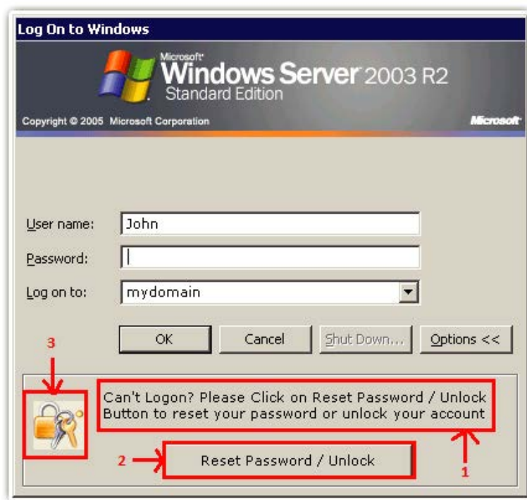
Figure 1. Frame text, button text, and icon for Windows XP/Windows Server 2003 and below.
