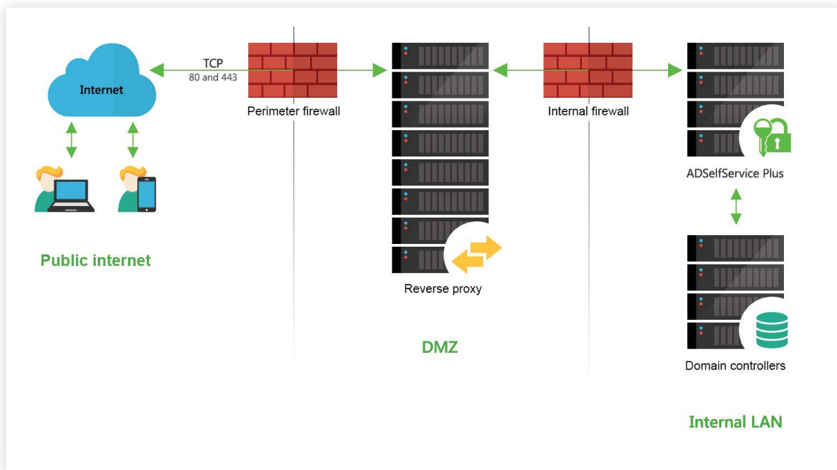
Figure 1: A reverse proxy server in a DMZ, while the ADSelfService Plus server is hosted in the intranet.
