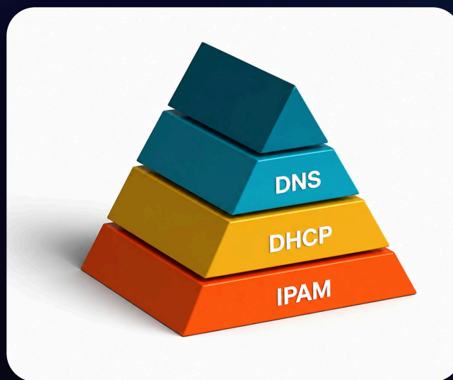
Figure 4 — DDI as a stack: IPAM is the foundation (which addresses exist and who owns them), DHCP sits above it (who gets one, and with what settings), and DNS sits on top (what name points where).
